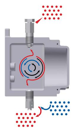
The sole installation of valve on bottom with the combined function of drain and breather is giving, anyway, a good result and, since the water penetration is practically impossible due to installation point, the IP X6 protection is guaranteed also with the UVD model (always open).
